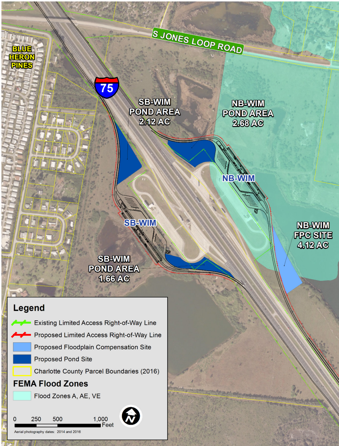
Figure 6-3: NB & SB WIM Rest Area Sites
